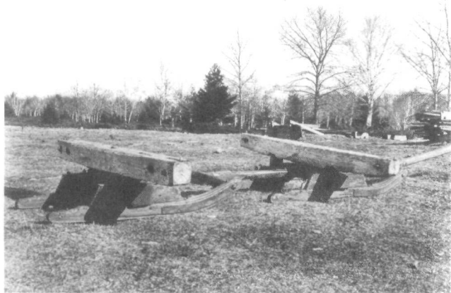
Fig. 8. A one-beam sleigh used for hauling sawlogs, ca. 1880s. (Photo: PAC, neg. no. C-30531.)
