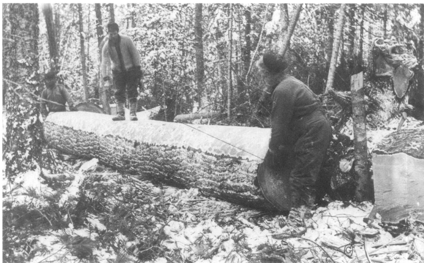
Fig. 6. The liner pulled the chalk line taut and let it snap against the timber, marking a line which was used by scorers and hewers to complete squaring the timber. (Photo: PAC, neg. no. PA-121801.)
